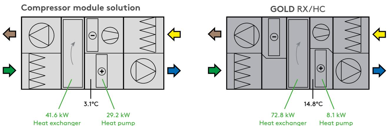
This shows that compressor module solutions largely have to heat the supply air via the heat pump. In the GOLD RX/HC, however, the rotary heat exchanger meets a higher proportion of the power requirement by recovering heating energy from the extract air, which is basically cost-free electrical energy. The heat pump can then top up the remaining proportion of the heating requirement.
