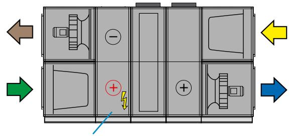
Electrical air heater placed in RX/HC (accessory)
