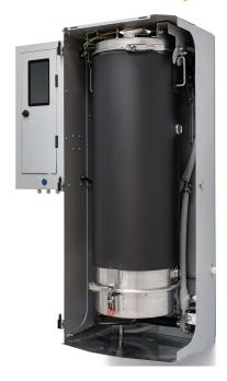
**ISE** steam exchange humidifier by **steamOvap®** is using energy from a central boiler pressurized steam or high temperature hot water to produce pure and sterile steam that is easy to distribute in air handling unit or ventilation duct.
