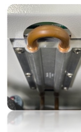
Refrigerant cooling of the compressor driver
