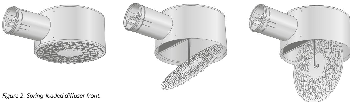
Figure 2. Spring-loaded diffuser front.
