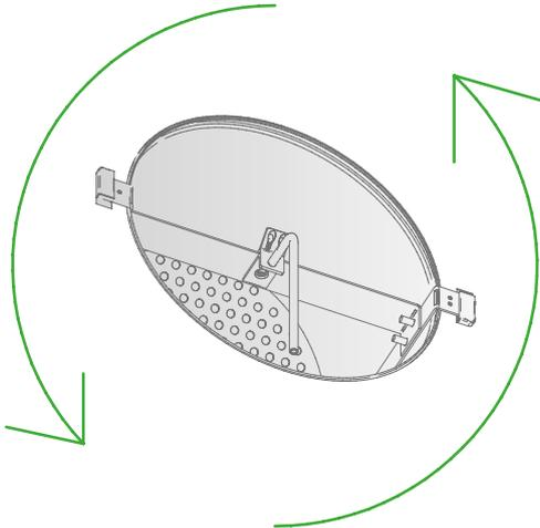
*The damper is turned anticlockwise and pulled out.*
